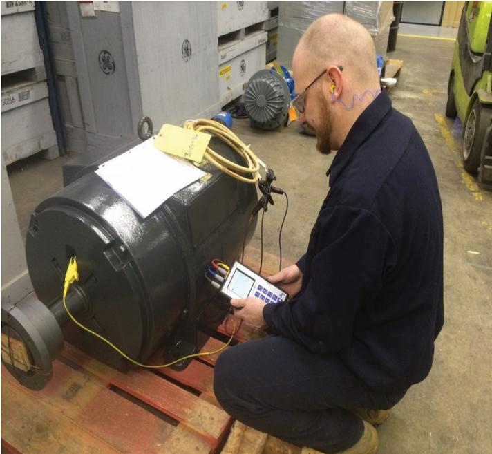
*Koontz-Wagner Service Technician, Erik Lehman, utilizes the ALL-TEST PRO 5™ to perform initial inspection of a 50HP motor in the repair shop.*
